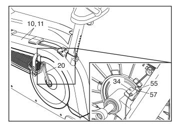
See the lower drawing at the left. Carefully pull the tops of the Shields (10, 11) apart and locate the Reed Switch (57). Rotate the Left Crank Arm (20) until a Magnet (55) is aligned with the Reed Switch. Then, slightly loosen the M4 x 18mm Truss Screw (34), slide the Reed Switch slightly toward or away from the Magnet, and then retighten the Truss Screw.
