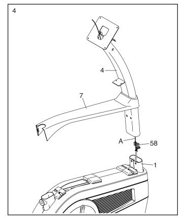
5. **Tip: Avoid pinching the wires.** Slide the Upright (4) onto the Frame (1).
