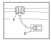
It may take some time for the console to be ready for use. IMPORTANT: In an emergency, the key can be pulled from the console, causing the walking belt to slow to a stop. Test the clip by carefully taking a few steps backward; if the key is not pulled from the console, adjust the position of the clip.
