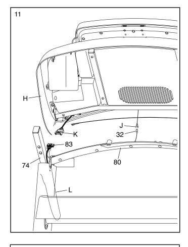
12. Attach the console assembly (H) to the Handrails (74) with four 5/16" x 2" Screws (2) and four 5/16" Star Washers (8); start all four Screws, and then tighten them. Be careful not to pinch the wires (K).
