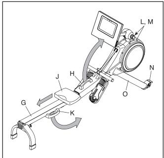
Next, hold and lift the Frame Handle (H) and the Rail Handle (K), and tip the rower forward onto the Shields (L, M) and the Storage Feet (N) (see the drawing on page 13).
