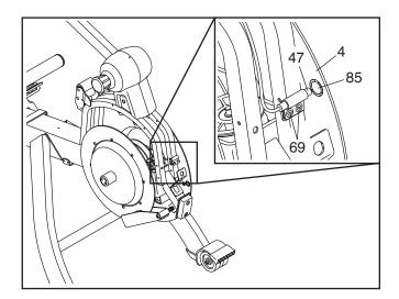
Turn the Left Flywheel (4) so that the Magnet (85) passes the Reed Switch (47) repeatedly. Repeat these actions until the console displays correct feedback.
