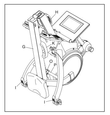
To unfold the rower, first place your foot on a Stabilizer Foot (I) and pull the Rail Handle (K) outward to disengage the Folding Clamp (O).
