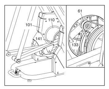
When you have properly adjusted the Drive Belt A (61), reattach the Access Cover (110) and plug in the power cord.
