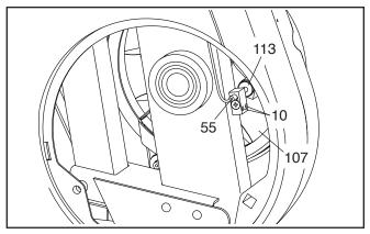
Then, slightly loosen the two M4 x 25mm Screws (10) and slide the Reed Switch (55) slightly closer to or away from the Magnet (113).
