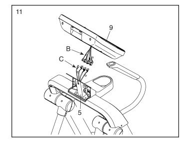
12. **Tip: Avoid pinching the wires.** Attach the Console (9) to the Console Bracket (5) with four M4 x 16mm Screws (141); **start all the Screws, and then tighten them.**
