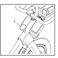
cycle, loosen the brake knob.
