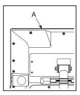
power switch and unplug the power cord. Next, locate the small reset opening (A) on the top of the console.
