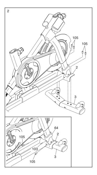
Attach the Rear Stabilizer (4) to the Base (2) with four M10 x 20mm Screws (105); do not fully tighten the Screws yet.
