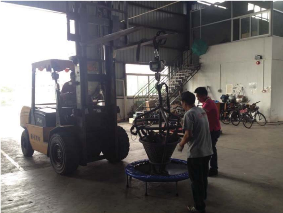
Picture 3 : Bed deflection and strength test
