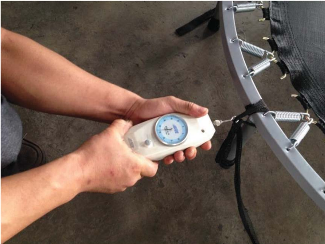
Picture 11 : connection strength of the legs test
