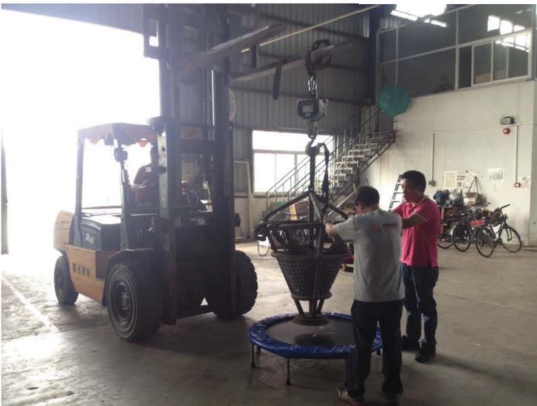
Picture 2 : Bed deflection and strength test
