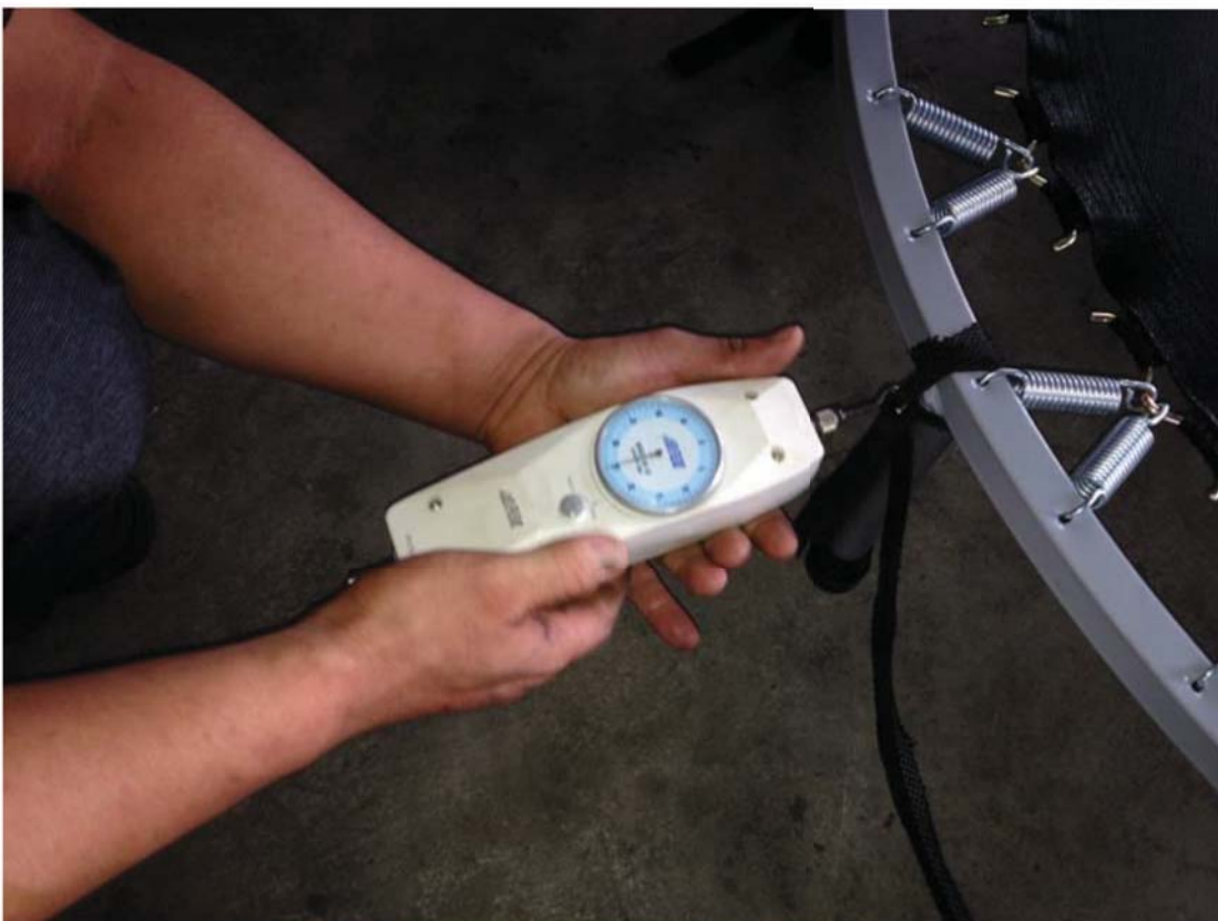
Picture 10 : connection strength of the legs test
