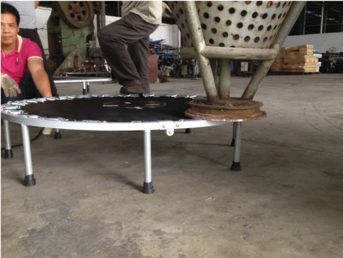
Picture 9 : stability test
