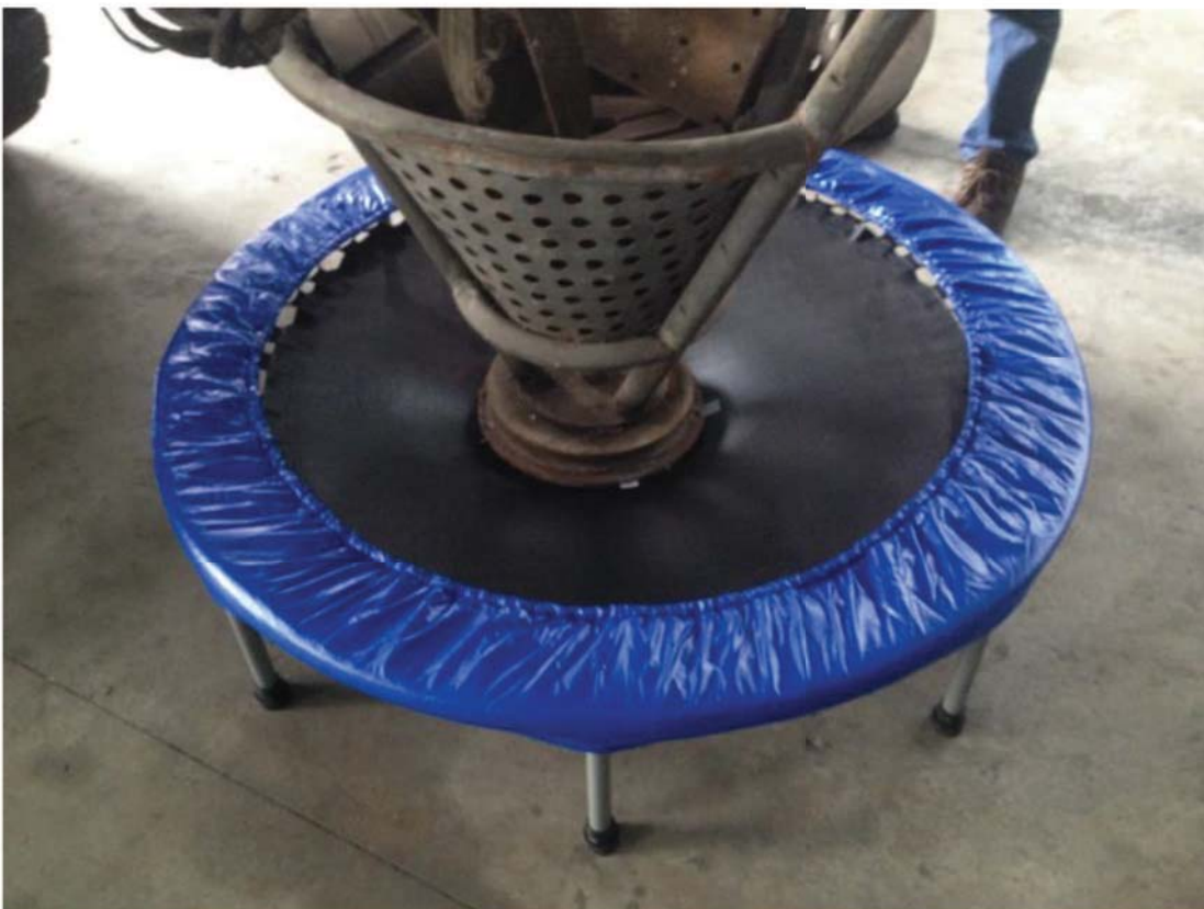
Picture 4 : Bed deflection and strength test
