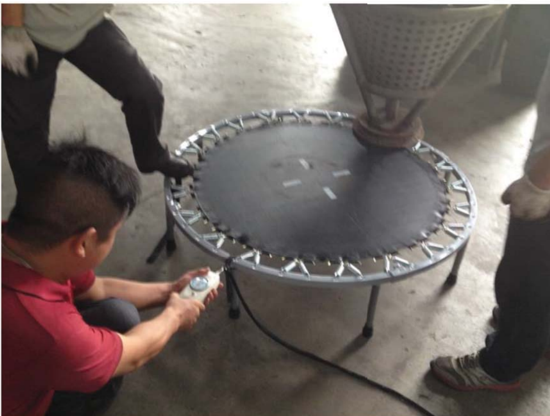
Picture 12 : connection strength of the legs test
