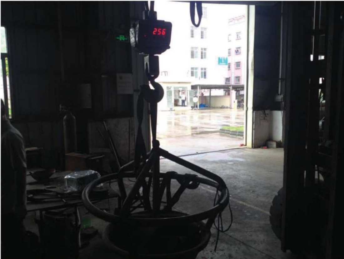
Picture 1 : Bed deflection and strength test
