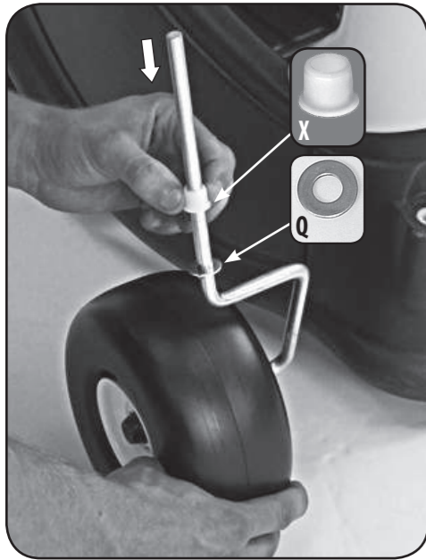
Slide washer, then bushing onto assembled right axle. Repeat on left axle.
