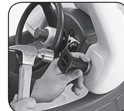
Place axle cap tool over ignition base and hammer. Snap on ignition top.
