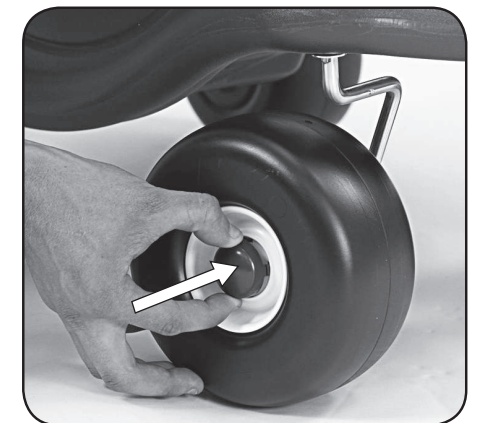
Align slots and snap on center caps.
