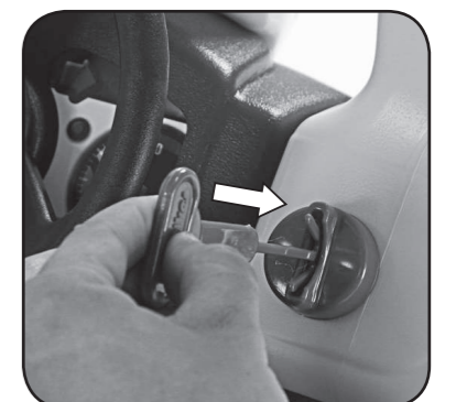
Squeeze the end of key to push through ignition base.
